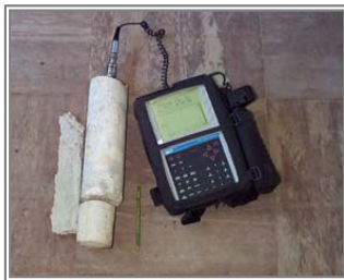
FIGURE 4 The collector-analyzer CMVA55 was used. Sensor is glued on one end of the specimen
